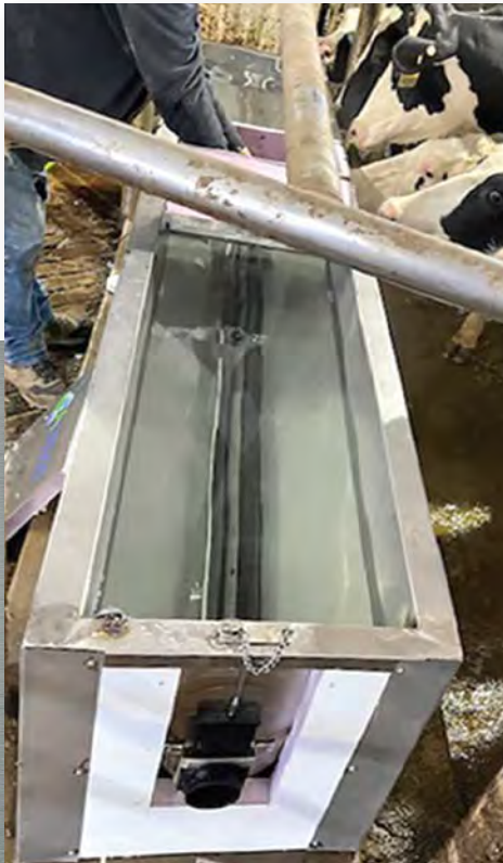
Step 2: Baffle plate closed.
